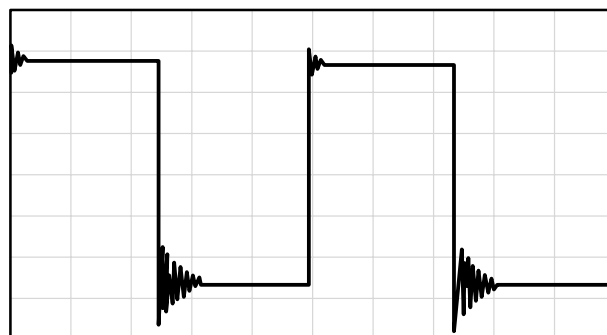
(b) C_L = 130 \text{ pF} , R_L = \text{NO LOAD}
